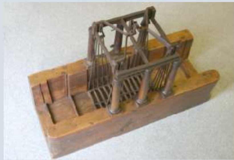
Model of the Brimscombe boat weighing machine - made in 1843 to demonstrate proposed mechanism
